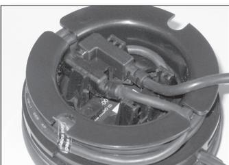
With the cradle installed it is now possible to install the antenna. Clip the extension to the antenna cable and lock the two in place using the tabs inside of the base. There is only one way the base can be inserted into the cradle, so make note of the position of the slot. Insert the base into the cradle and twist to lock.
