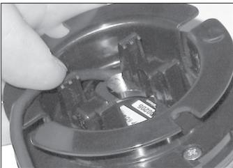
This step requires the two machine screws provided with the Antenna Dock. First, run the antenna cable through the inside of the base. Capture the cable with the slot at one end of the base. This will allow the base to sit flush against the antenna.
